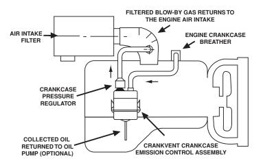
A crankcase ventilation filter should be made below the valve cover but above the oil pan.
